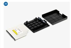
3. Assemble the OWC Slim back together without a drive by aligning the top with the bottom-back. Press down while moving from back-to-front. The top and bottom will snap back together.
